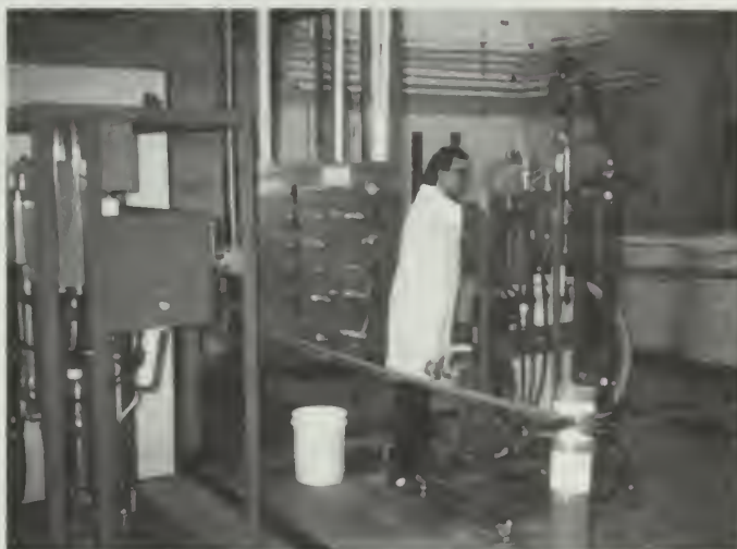
FIGURE 5-6: THE ULTRAFILTRATION UNIT, SET UP IN HWRIC'S PILOT LAB
